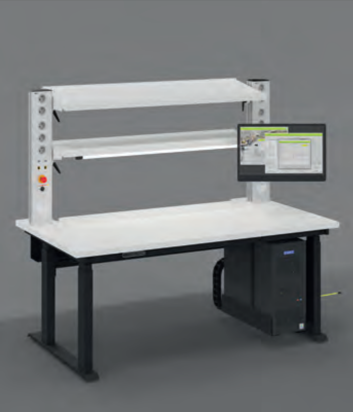
Fig. 2: Expanding profile 2 straight towards the user, version 2: ELC.B2.A2 with shelves for table type Basic 2, ELC3.4.1631.B (order no. Expanding profile 2, see from page 129). Optionally with PC holder for steel table frame and LED-ProSlim system light mounted under the shelf.
