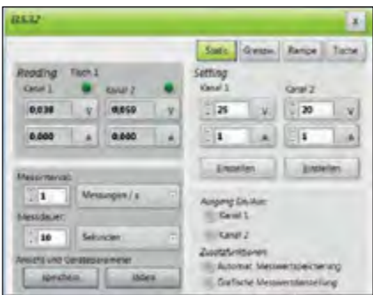
Example of a DC source: power supply unit with voltage and current limiting ( U_{max} and I_{max} ) and automatic data storage.
