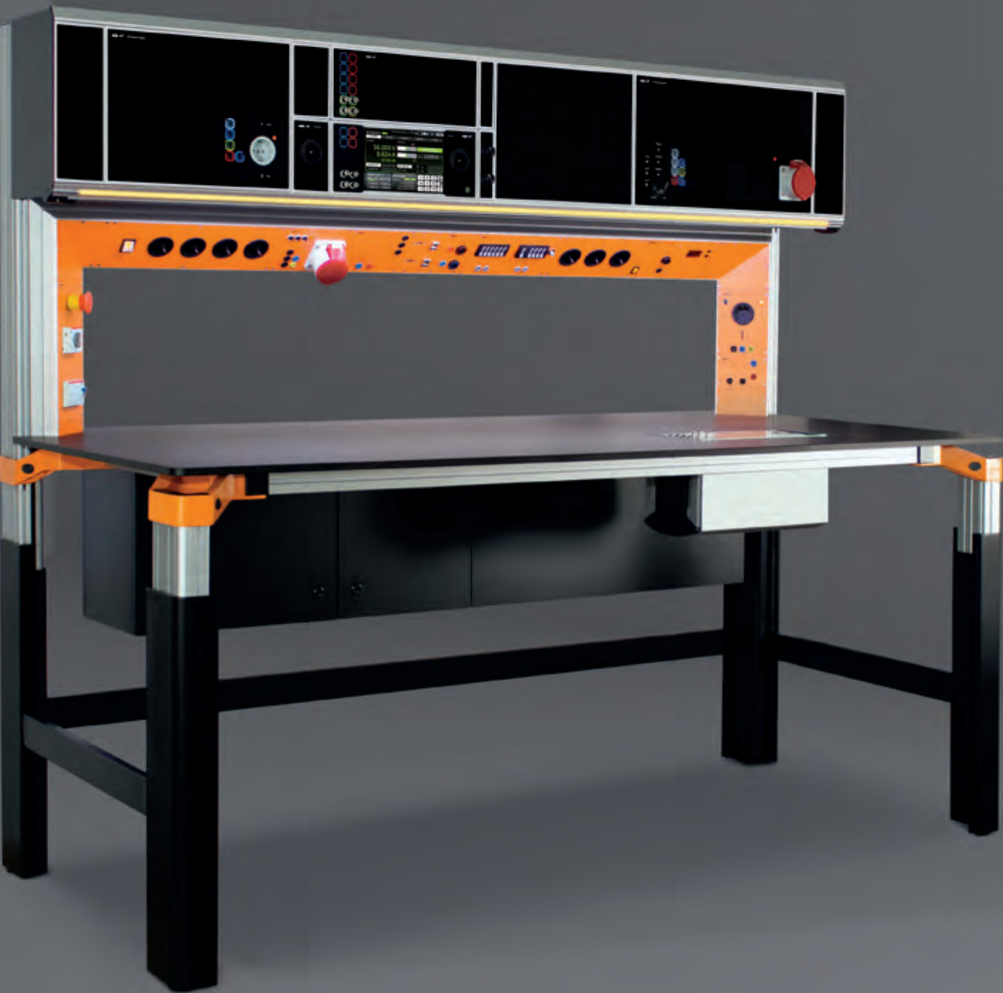
Figure 1: Table with 19-inch / 6 U cockpit. Invisibly integrated LED workstation lighting and integrated RGB indication light across the entire width of the laboratory bench (options). Table top equipped with the elneos six appliance series (complete glass appliance front).
