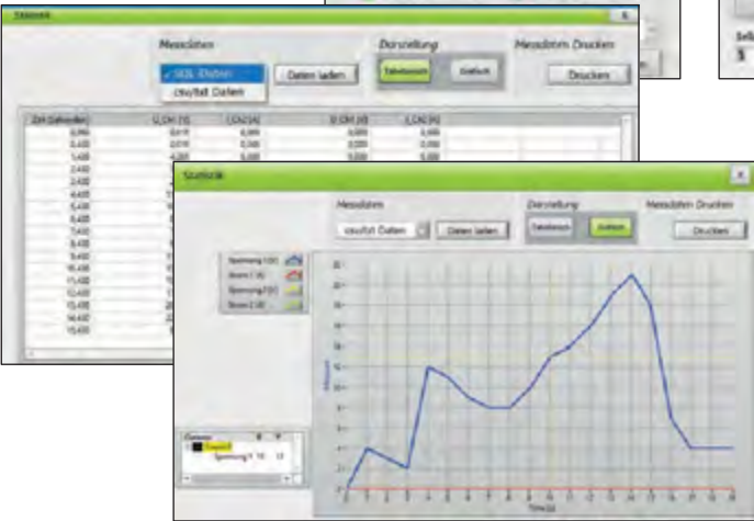
Examples: Graphical and tabular display of measured values. The measurement data is visualized in a table and simultaneously in a graphic during the measurement process. An HTML report for an Internet browser is created via a command.
